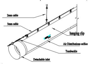
Double row suspension is recommended for ducts with diameter larger than 500 mm (20"). Cable and accessories include 5mm plastic coated galvanized cable, eye bolts, turnbuckles, cable clamps, 2mm mid-supporting cable shall be supplied by fabric duct manufacturer. Mounting bracket at both ends of tension cables shall be supplied by contractor.
