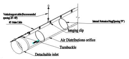
Option 4 URR (Uniform air velocity Conic Duct with Internal Retention Ring) system with Galvanized Tension Cable suspension
