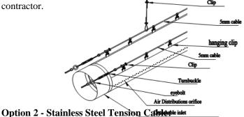
a) Suspension system consists of one row or two rows or multi-rows of plastic coated galvanized cables located 50mm to 90mm (2" to 4") above fabric duct mounting points. Mounting points shall locate at 12 o'clock (for single row suspension), and 10, 2 o'clock for double row suspension, or specified multi-rows o'clock positions for rectangular duct. Distance between clips shall not exceed 500 mm (20").
