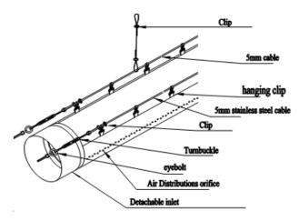
Option 3 IRR (Internal Retention Ring) system with Galvanized Tension Cable suspension
